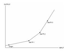
If an origin and 3 points had been programmed then between these points the output would follow the profile and the centre LED will flash about once per second. If the input goes past either the Origin or, in this case, Set Pt 3, the unit will extrapolate a linear output using the last gradient calculated and a 'o' ('o'ut of range) will appear in the display.
