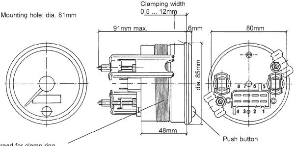
Thread for clamp ring (clamping width 0.5 ... 12mm or 12 ... 23mm)
