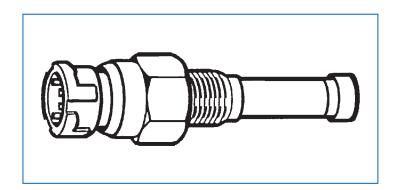
If the vehicle is already equipped with a speed sensor. Request a data sheet of this sensor. Ask your vehicle manufacturer or VDO Kienzle whether the speed sensor can be used.
