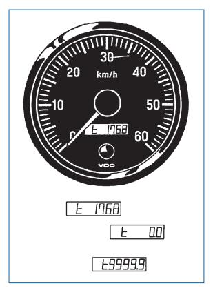
Trip and total distance remain stored after the operating voltage is switched off.
