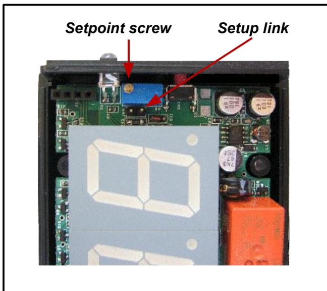
Identify the setpoint adjust screw and setup link
