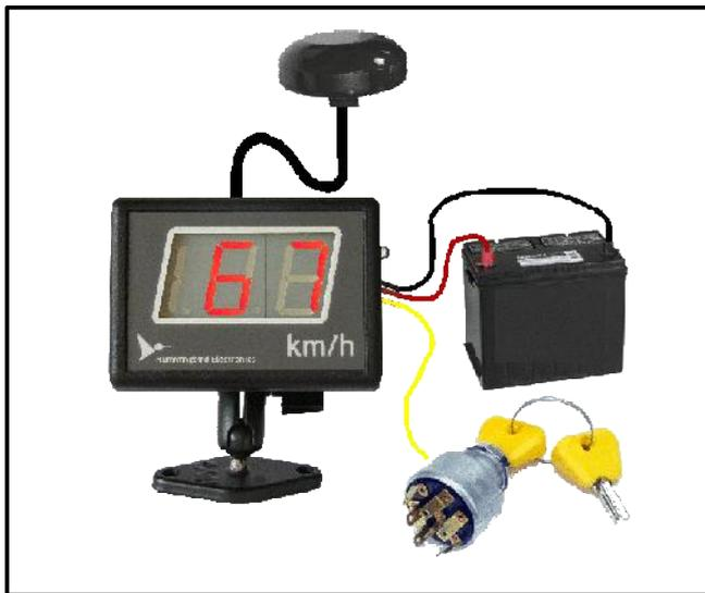
Typical GPS Speedometer installation
