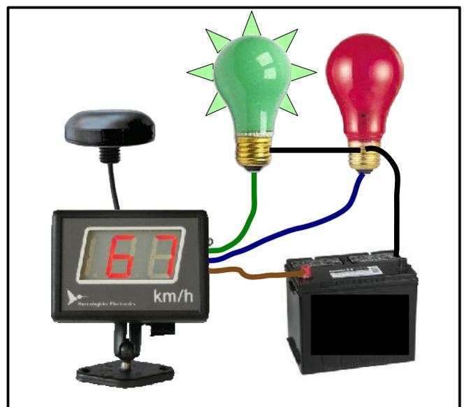
Typical speed switch installation – the green light (connected to normally-closed) will be on until the speed setpoint is exceeded at which point the red light will be on and the green off.
