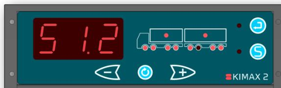
When you press
