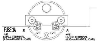
Connect to Vehicle Chassis (Battery Pos)
